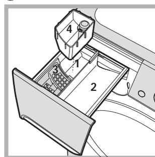
This function is particularly useful for the removal of stubborn stains. Insert extra compartment 4 (supplied with the appliance) into compartment 1. When pouring in the bleach, be careful not to exceed the "max" level marked on the central pivot (see figure). To bleach laundry with no other washing action, pour the bleach
